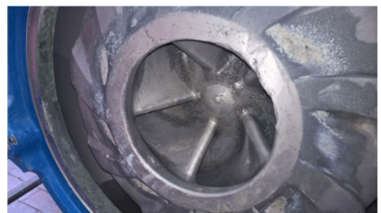
Close inspection shows no significant wear during the test period
